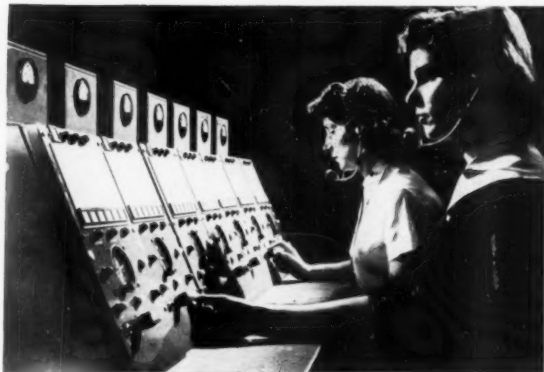
RELAY OPERATORS (left) who transmit Volscan flight path instructions may soon be replaced by automatic voice relay. Voice recordings of key word-groups stored on magnetic drum (above), are automatically pieced together according to Volscan signals to form complete voice commands which are then transmitted over UHF/VHF radio channels.
